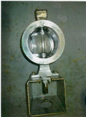
With Zirolflex Coating – Minimum Wear visible
