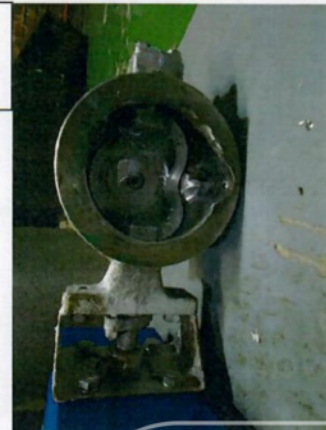
Without Zirolflex Coating – Aggressive Wear visible
