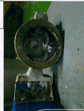
Without Zirotflex Coating – Aggressive Wear visible
