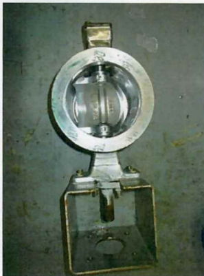
With Zirotflex Coating – Minimum Wear visible
